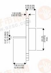
Bipolar PNP Device in a Hermetically sealed TO3 Metal Package.
