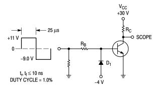
$R_B$  and  $R_C$  VARIED TO OBTAIN DESIRED CURRENT LEVELS D1 MUST BE FAST RECOVERY TYPE, e.g.: 1N5825 USED ABOVE  $I_B\approx 100$  mA MSD6100 USED BELOW  $I_B\approx 100$  mA
