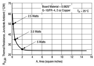
Figure 14. Thermal Resistance versus Collector Pad Area for the D<sup>2</sup>PAK Package (Typical)
