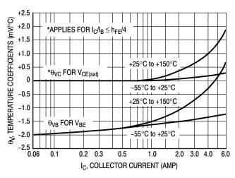
Figure 11. Temperature Coefficients
