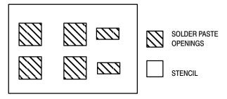
Figure 15. Typical Stencil for DPAK and D<sup>2</sup>PAK Packages
