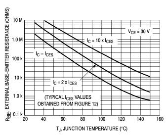
Figure 13. Effects of Base-Emitter Resistance
