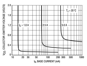
Figure 9. Collector Saturation Region
