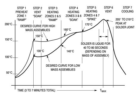
Figure 16. Typical Solder Heating Profile
