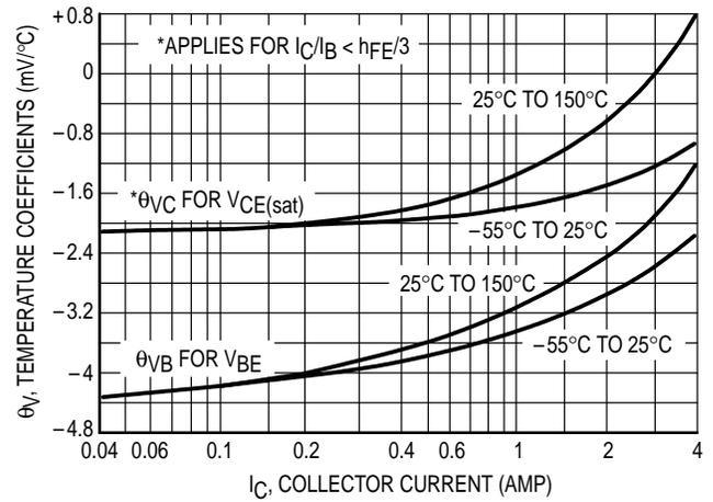
Figure 10. Temperature Coefficients
