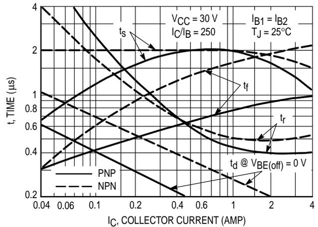
Figure 2. Switching Times
