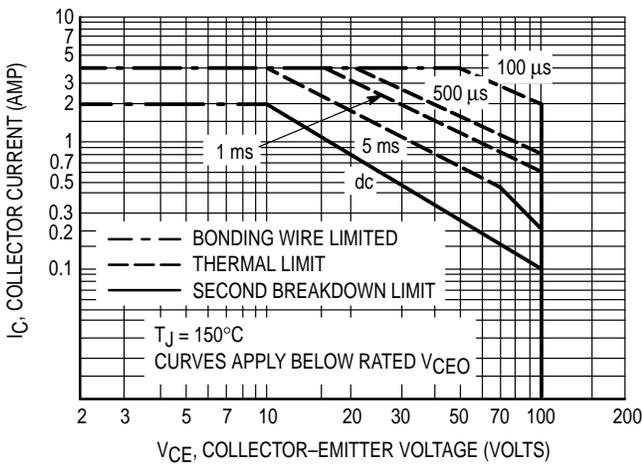
Figure 4. Maximum Rated Forward Biased Safe Operating Area
