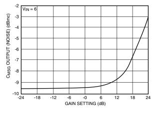
Figure 5. C<sub>MSG</sub> Output Noise vs Gain Settings
