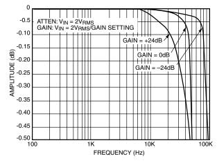
Figure 3. Amplitude vs Frequency (VIN/VOUT = 2VRMS)
