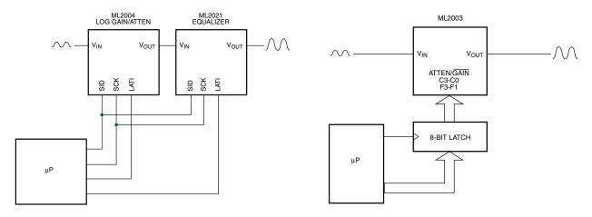
Figure 12. Typical Serial Interface
