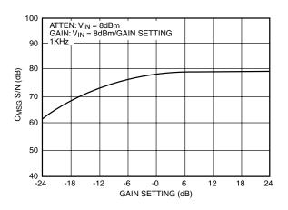
Figure 6. C<sub>MSG</sub> S/N vs Gain Setting
