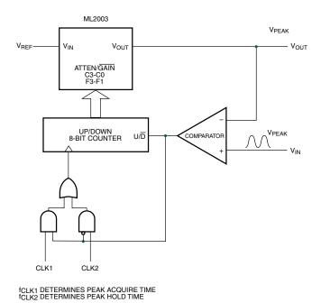
Figure 18. Precision Peak Detector (±1%) with Controllable Acquire and Hold Time
