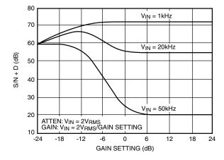
Figure 8. S/N + D vs Gain Setting (VIN/VOUT = 2VRMS)
