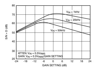
Figure 9. S/N + D vs Gain Setting (VIN/VOUT = 0.5VRMS)
