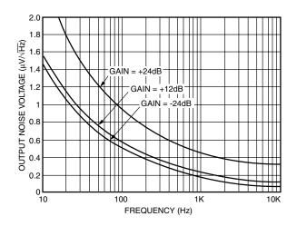
Figure 4. Output Noise Voltage vs Frequency
