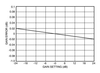
Figure 7. Gain Error vs Gain Setting
