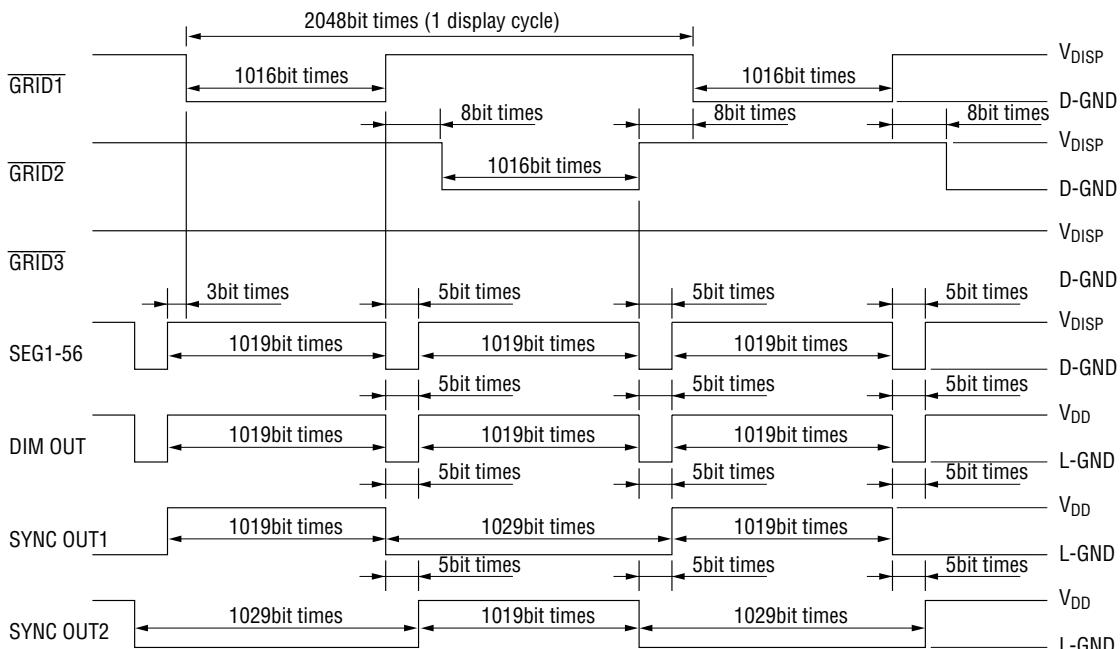
● **Output Timing (Triplex Operation)** \*1bit time=4/f<sub>OSC</sub>
