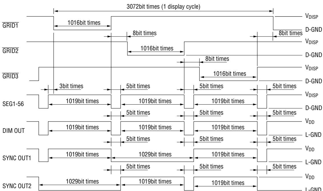
● **Output Timing (Duplex Operation)** \*1bit time=4/f<sub>OSC</sub>
