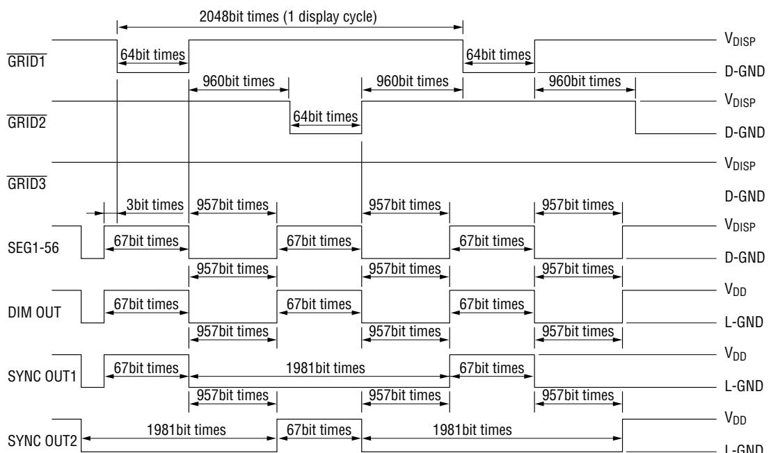
● **Output Timing (Triplex Operation)** \*1bit time=4/f<sub>OSC</sub>
