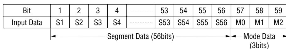
[Bit correspondence between segment output and segment data]
