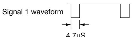
\*3 Measuring horizontal sync signal pull-in range
