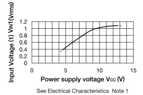
7. Input voltage (2) - Power supply voltage (QSrround)
