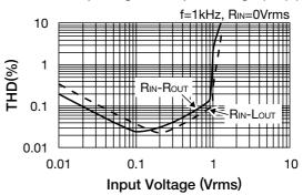
THD of output signal – Input voltage (QSrround f=1kHz, The signals that are inputted in LIN and RIN are out out of phase and same amplitude.
