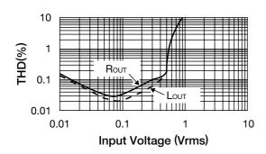
5. THD of output signal - Input voltage (QSrround) 6. Input voltage (1) - Power supply voltage (QSrround)
