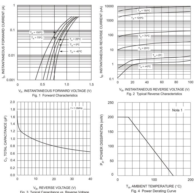
Fig. 3 Typical Capacitance vs. Reverse Voltage
