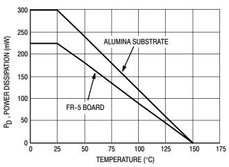
Figure 4. Steady State Power Derating Curve
