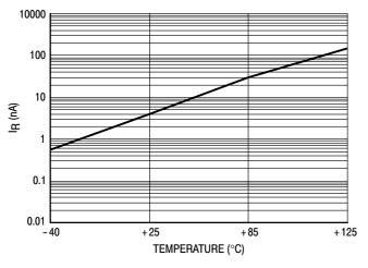
Figure 3. Typical Leakage Current versus Temperature
