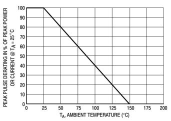
Figure 6. Pulse Derating Curve
