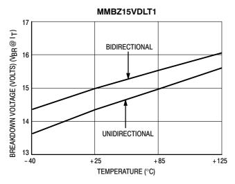
Figure 1. Typical Breakdown Voltage versus Temperature
