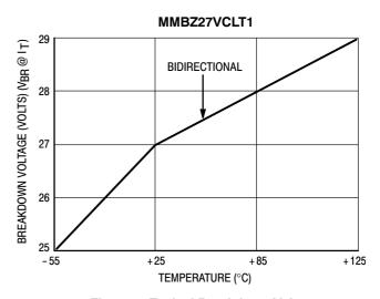
Figure 2. Typical Breakdown Voltage versus Temperature
