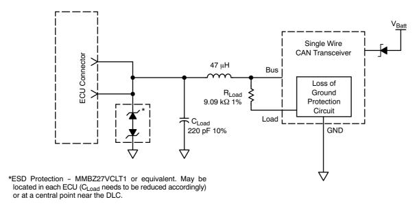
Figure 7. Single Wire CAN Network
