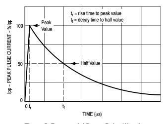
Figure 5. Exponential Decay Pulse Waveform
