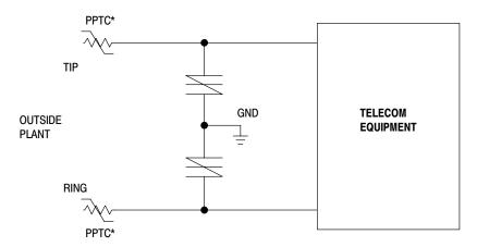
\*Polymeric PTC (positive temperature coefficient) overcurrent protection device
