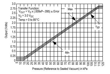
Figure 4. Output versus Pressure Differential
