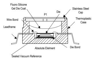
Figure 2. Cross Sectional Diagram SSOP (not to scale)
