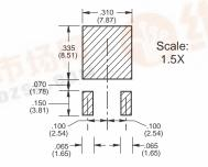
**Soldering Note:** During surface mount soldering the soldering temperature profile must not cause the metal tab of this device to exceed 220°C.
