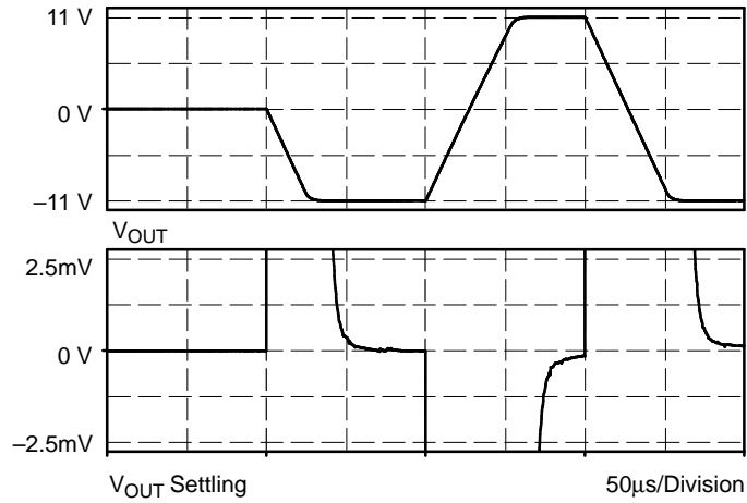
Graph 1. Typical Output Settling Characteristic V_{REF} = 5\text{ V} , R_L = 5\text{ K} , C_L = 500\text{ pF}
