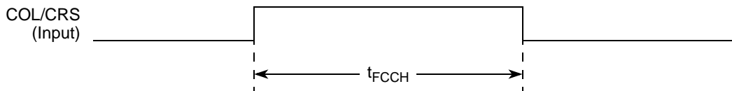
Figure 26. Ethernet Collision AC Timing Diagram (FCC)
