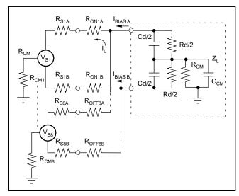
FIGURE 2. MPC507A Static Accuracy Equivalent Circuit.
