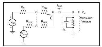
FIGURE 1. MPC506A Static Accuracy Equivalent Circuit.
