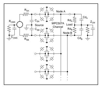
FIGURE 4. Settling and Common-Mode Effects—MPC507A
