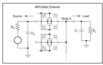
FIGURE 3. Settling Time Effects—MPC506A.
