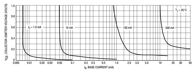
Figure 4. Collector Saturation Region
