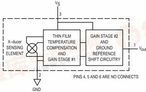
Figure 1. Fully Integrated Pressure Sensor Schematic
