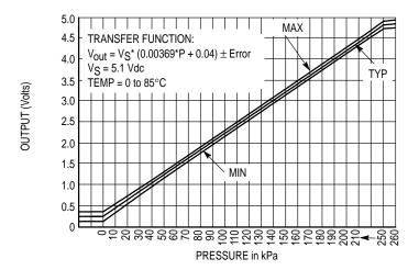
Figure 4. Output versus Differential Pressure
