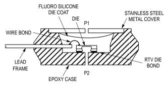
Figure 2. Cross-Sectional Diagram (Not to Scale)
