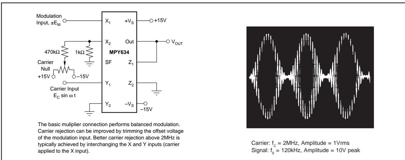
FIGURE 11. Balanced Modulator.
