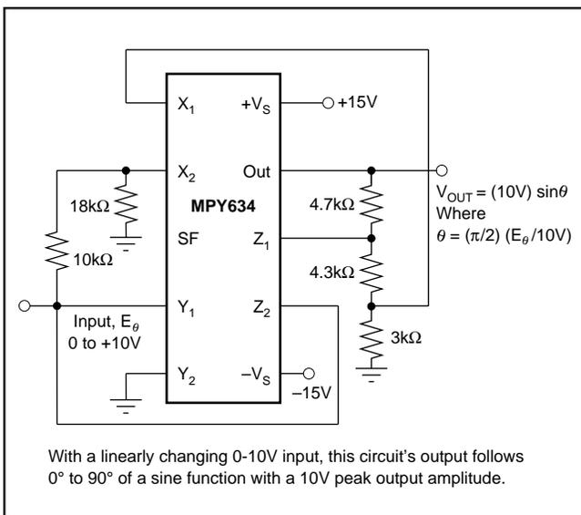
FIGURE 8. Sine-Function Generator.
