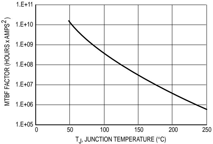
This above graph displays calculated MTBF in hours x ampere<sup>2</sup> emitter current. Life tests at elevated temperatures have correlated to better than  $\pm 10\%$  of the theoretical prediction for metal failure. Divide MTBF factor by  $I_C^2$  for MTBF in a particular application.
