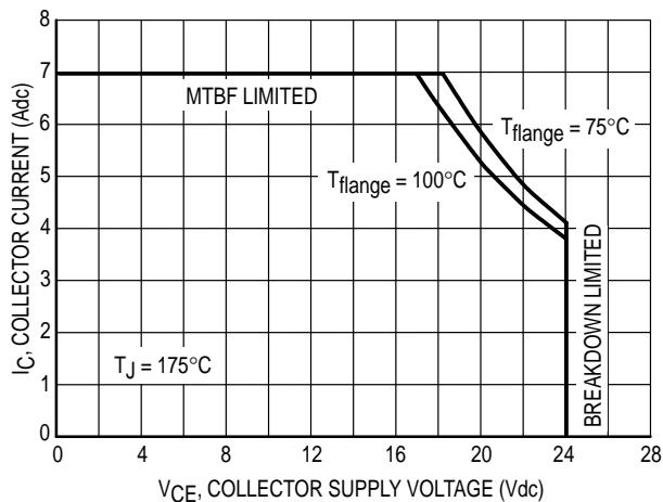
**Figure 9. Class A DC Safe Operating Area**
