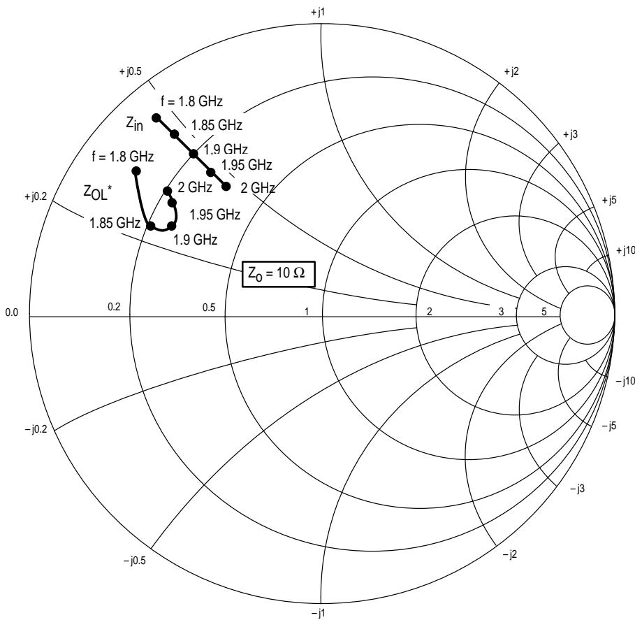
$V_{CC} = 26 \text{ V}$ ,  $I_{CQ} = 200 \text{ mA}$ ,  $P_{out} = 60 \text{ W (PEP)}$
