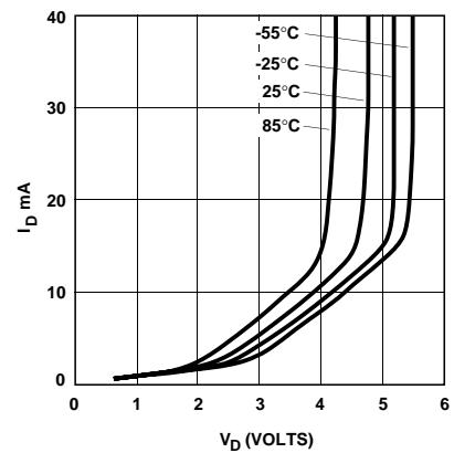
Figure 6.  $I_D$  vs.  $V_D$  at Four Temperatures.
