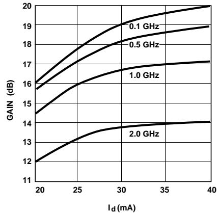
Figure 2. Power Gain vs. Current at 25°C.
