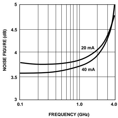
Figure 4. Noise Figure vs. Frequency at  $I_D = 32$  mA.
