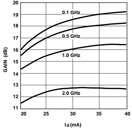
Figure 2. Power Gain vs. Current at 25°C.
