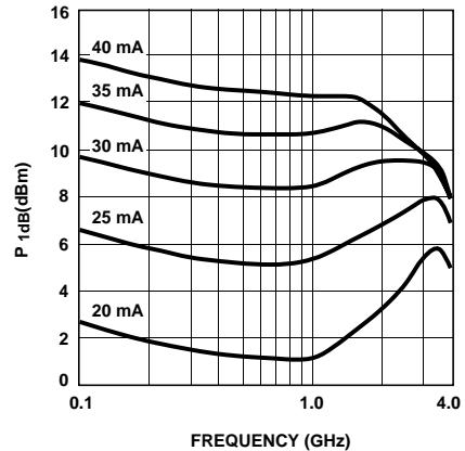
Figure 3. Typical  $P_{1dB}$  vs. Frequency at 25°C.
