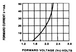
Fig.1 FORWARD CURRENT VS. FORWARD VOLTAGE.
