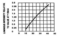
IF-FORWARD CURRENT-MA Fig.3 RELATIVE LUMINOUS INTENSITY VS. FORWARD CURRENT
