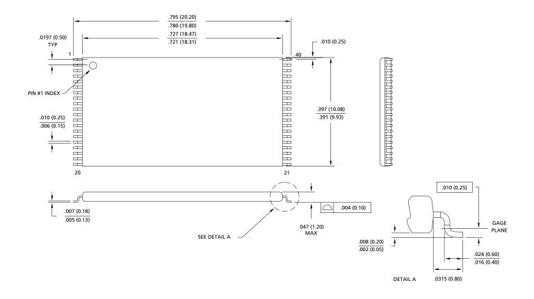
NOTE: 1. All dimensions in inches (millimeters) MAX/MIN or typical where noted.
