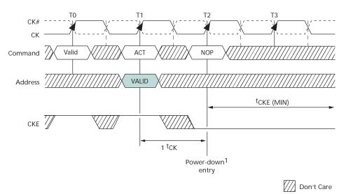
Notes: 1. The earliest active power-down entry may occur is at T2, which is 1 × <sup>t</sup>CK after the ACTI-VATE command. Active power-down entry occurs prior to <sup>t</sup>RCD (MIN) being satisfied.
