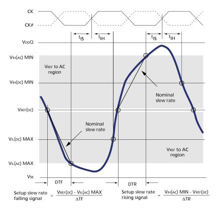
Figure 26: Tangent Line for <sup>t</sup>IS
