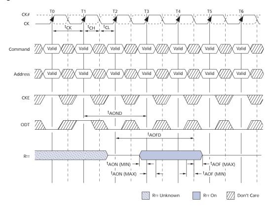
Figure 86: ODT Timing for Slow-Exit or Precharge Power-Down Modes
