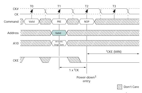
Notes: 1. The earliest precharge power-down entry may occur is at T2, which is 1 × <sup>t</sup>CK after the PRE-CHARGE command. Precharge power-down entry occurs prior to <sup>t</sup>RP (MIN) being satisfied.
