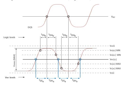
Figure 36: AC Input Test Signal Waveform (Differential)
