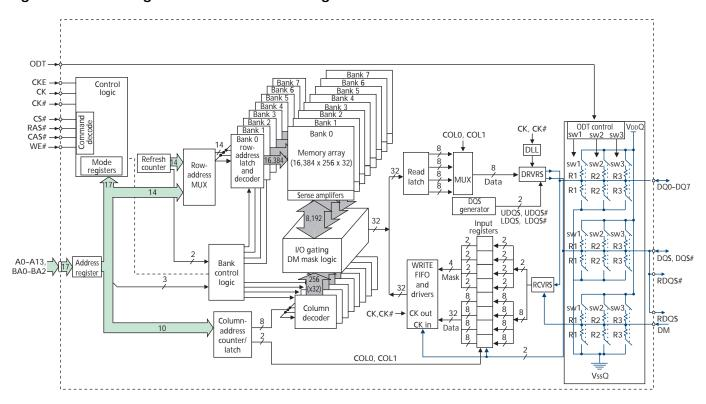
Figure 5: 64 Meg x 16 Functional Block Diagram
