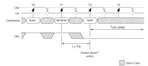
Notes: 1. The earliest precharge power-down entry may occur is at T2, which is 1 × <sup>t</sup>CK after the REFRESH command. Precharge power-down entry occurs prior to <sup>t</sup>RFC (MIN) being satisfied.
