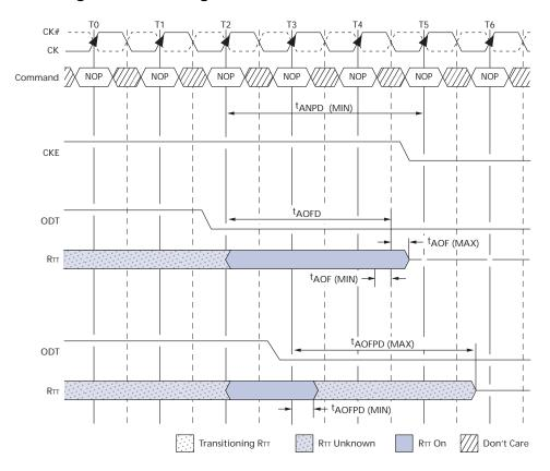
Figure 88: ODT Turn-On Timing When Entering Power-Down Mode
