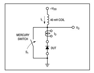
Figure 6. Test Circuit
