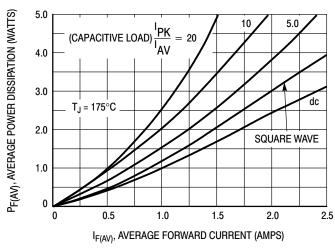
Figure 4. Power Dissipation
