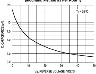
Figure 5. Typical Capacitance
