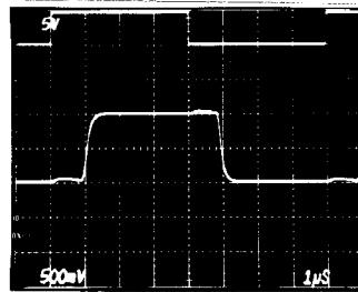
MUX-24 SMALL-SIGNAL SWITCHING WITH FILTERING
