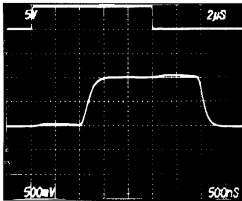
R_L = 1M\Omega, C_L = 500pF, V_1 = -700mV, V_g = +700mV
