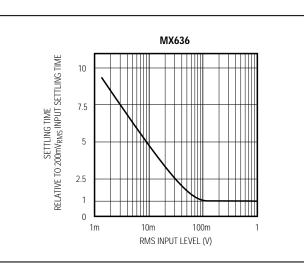
Figure 6b. MX636 Settling Time vs. Input Level
