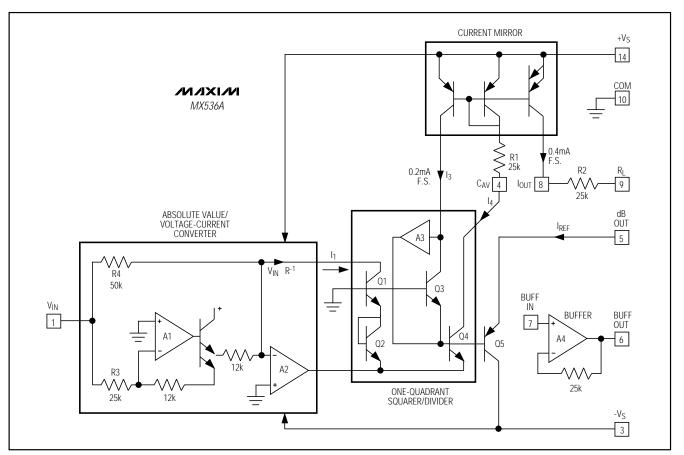
Figure 1. MX536A Simplified Schematic
