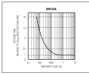
Figure 6a. MX536A Settling Time vs. Input Level
