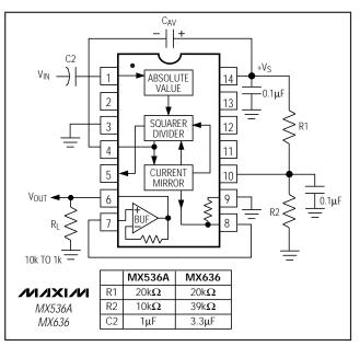
Figure 5. Single-Supply Operation
