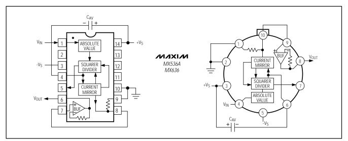
Figure 2. MX536A/MX636 Standard RMS Connection
