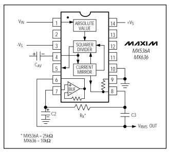
Figure 8. MX536A/MX636 with a Two-Pole Output Filter
