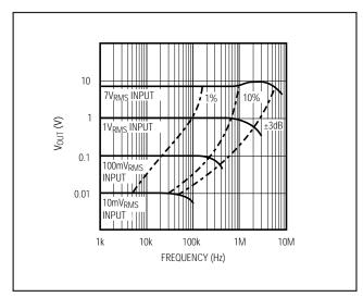
Figure 11. MX536A High-Frequency Response
