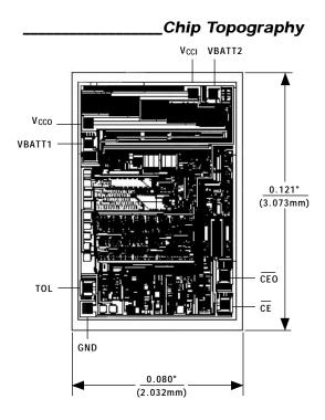
TRANSISTOR COUNT: 1436; LEAVE SUBSTRATE UNCONNECTED.
