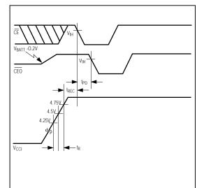
Figure 2. Power-Up Timing Diagram
