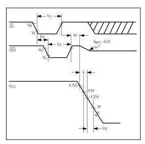
Figure 3. Power-Down Timing Diagram
