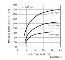
FIGURE 30. Maximum Load Current for Inverting Regulator Circuit
