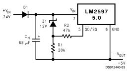
FIGURE 33. Undervoltage Lockout With Hysteresis for an Inverting Regulator
