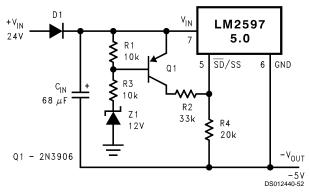
FIGURE 32. Undervoltage Lockout Without Hysteresis for an Inverting Regulator
