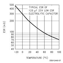
FIGURE 18. Capacitor ESR Change vs Temperature
