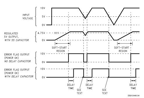
FIGURE 14. Timing Diagram for 5V Output
