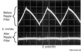
FIGURE 20. Post Ripple Filter Waveform
