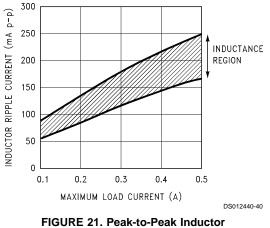
Ripple Current vs Load Current
