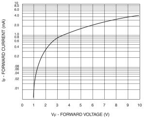
Fig. 3 Forward Voltage vs. Forward Current
