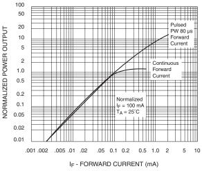
Fig. 1 Power Output vs. Input Current
