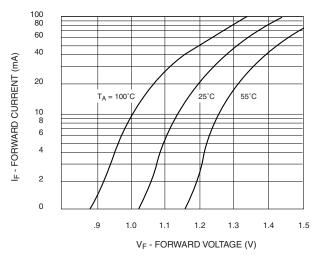
Fig. 4 Forward Voltage vs. Forward Current
