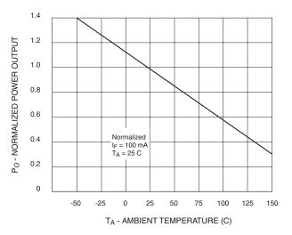
Fig. 2 Power Output vs. Temperature
