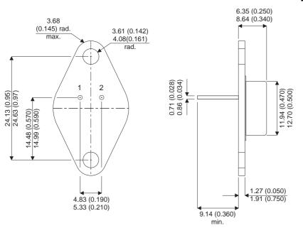
Bipolar NPN Device in a Hermetically sealed TO66 Metal Package.
