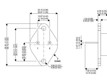
Bipolar NPN Device in a Hermetically sealed TO3 Metal Package.
