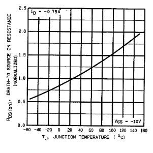
Fig 4. Normalized On-Resistance Vs. Temperature
