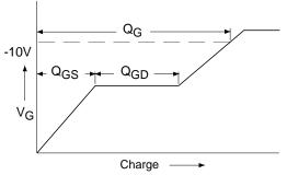
Fig 13a. Basic Gate Charge Waveform
