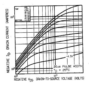
Fig 1. Typical Output Characteristics
