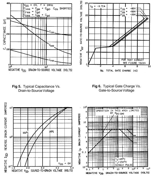
Fig 7. Typical Source-Drain Diode Forward Voltage Fig 8. Maximum Safe Operating Area
