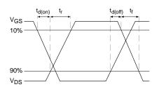
Fig 10b. Switching Time Waveforms
