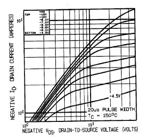
Fig 2. Typical Output Characteristics
