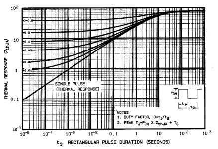
Fig 11. Maximum Effective Transient Thermal Impedance, Junction-to-Ambient
