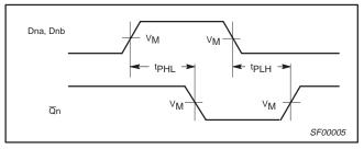
Waveform 1. Propagation delay for inverting outputs
