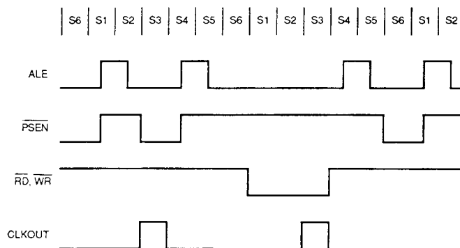
Figure 23. System Clock Timing Overview
