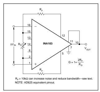
FIGURE 8. Use of External Resistors for Gain Set.
