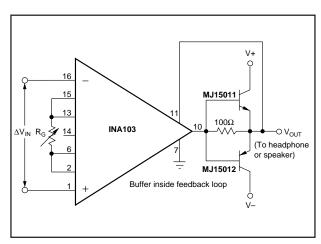
FIGURE 11. Increasing Output Circuit Drive.
