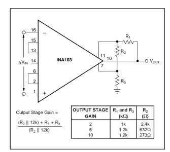
FIGURE 7. Gain Adjustment of Output Stage.
