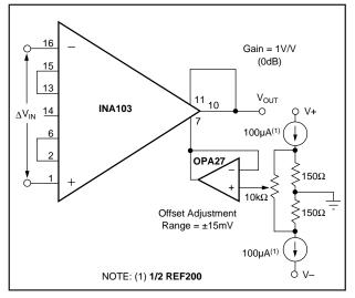
FIGURE 4. Output Offsetting.
