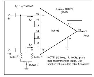
FIGURE 5. Input Offset Adjustment for AC-Coupled Inputs.
