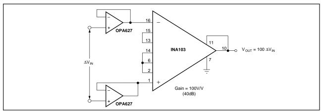
FIGURE 14. Gain-of-100 INA103 with FET Buffers.
