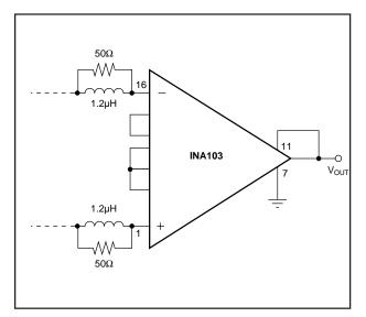
FIGURE 2. Input Stabilization Network.
