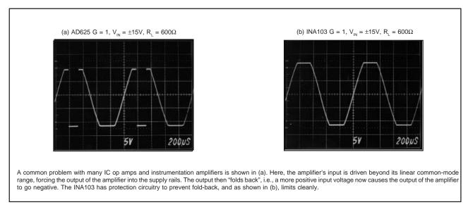
FIGURE 9. INA103 Overload Condition Performance.
