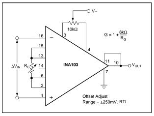
FIGURE 3. Offset Adjustment Circuit.
