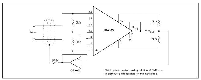
FIGURE 13. Instrumentation Amplifier with Shield Driver.
