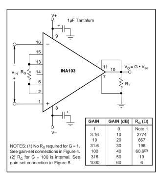
FIGURE 1. Basic Circuit Configuration.
