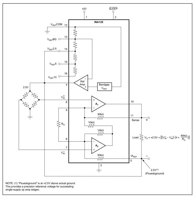
FIGURE 6. Psuedoground Bridge Measurement, 5V Single Supply.
