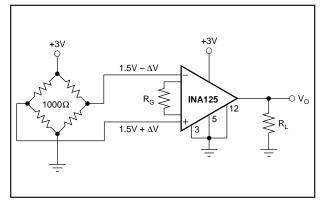
FIGURE 5. Single Supply Bridge Amplifier.
