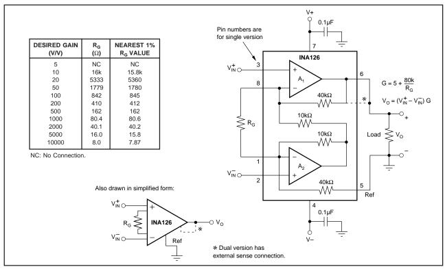
FIGURE 1. Basic Connections.
