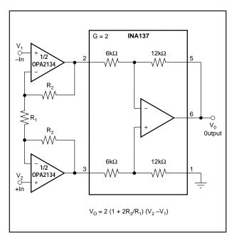
FIGURE 6. High Input Impedance Instrumentation Amplifier.
