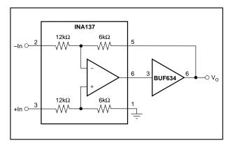
FIGURE 5. Boosting Output Current.
