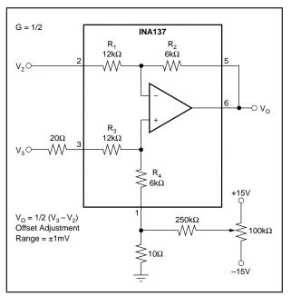
FIGURE 3. Offset Adjustment.
