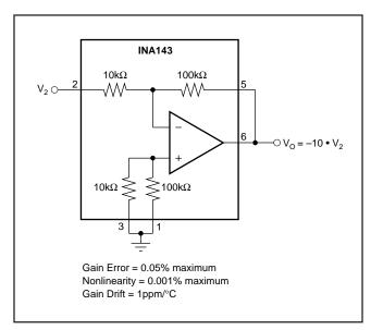
FIGURE 5. Precision G = -10 Inverting Amplifier.
