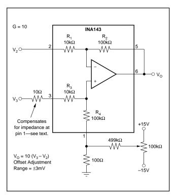
FIGURE 3. Offset Adjustment.
