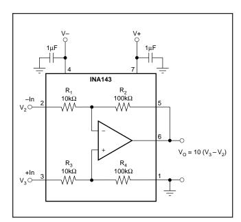
FIGURE 1. G = 10 Basic Power Supply and Signal Connections.
