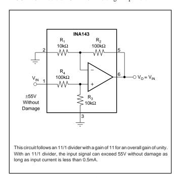
FIGURE 6. Voltage Follower with Input Protection.
