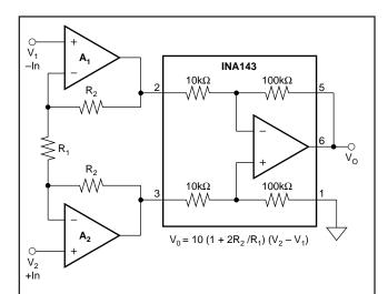
The INA143 can be combined with op amps to form a complete instrumentation amplifier with specialized performance characteristics. Burr-Brown offers many complete high performance IAs. Products with related performances are shown at the right in the table below.
