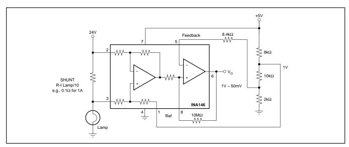
FIGURE 8. Comparator Output with Optional Hysteresis Application to Sense Lamp Burn-Out.
