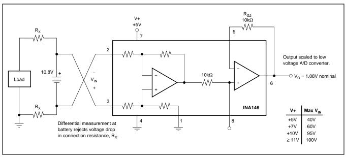
FIGURE 3. Measuring Voltages Greater than Supply Voltage.
