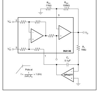
FIGURE 9. AC Coupling (DC Restoration).
