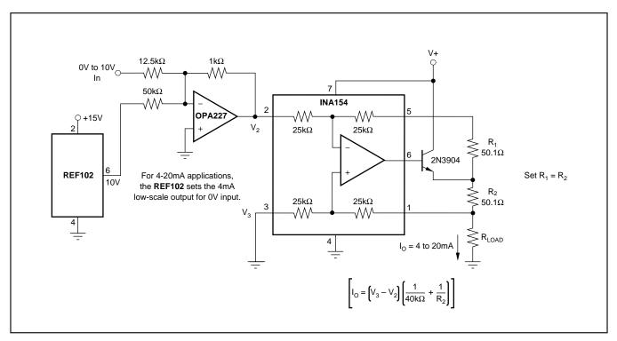
FIGURE 7. Precision Voltage-to-Current Conversion.
