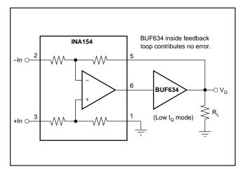
FIGURE 5. Boosting Output Current.
