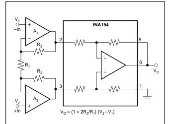
The INA154 can be combined with op amps to form a complete instrumentation amplifier with specialized performance characteristics. Burr-Brown offers many complete high performance IAs. Products with related performances are shown at the right.
