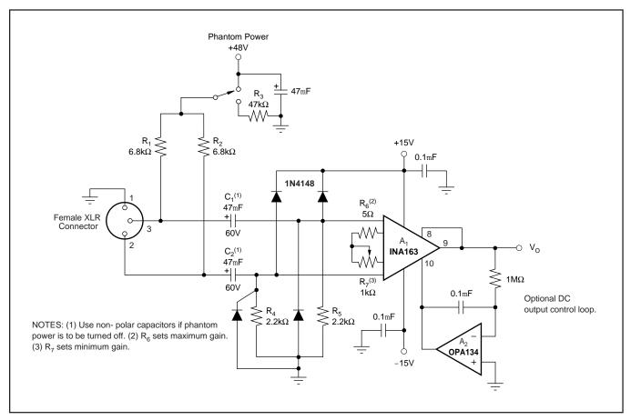
FIGURE 5. Phantom-Powered Microphone Preamplifier.
