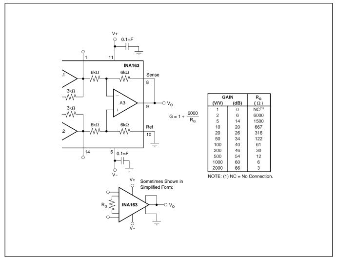
FIGURE 1. Basic Circuit Connections.
