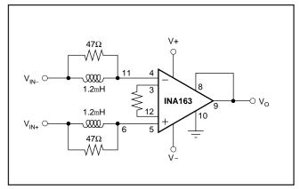
FIGURE 2. Input Stabilization Network.
