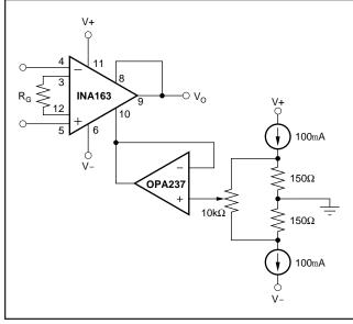
FIGURE 3. Offset Voltage Adjustment Circuit.
