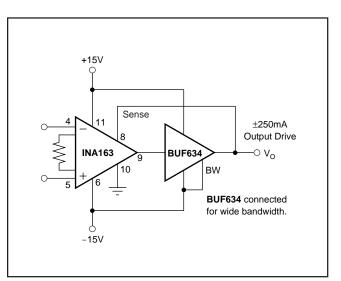
FIGURE 4. Buffer for Increase Output Current.
