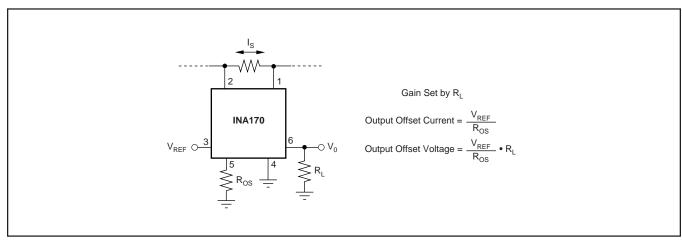
FIGURE 4. Offsetting the Output Voltage.
