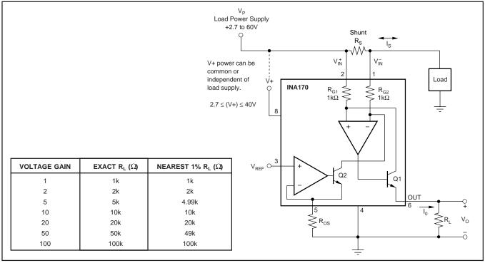
FIGURE 1. Basic Circuit Connections.
