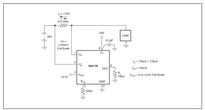
FIGURE 5. Bipolar Current Measurement.
