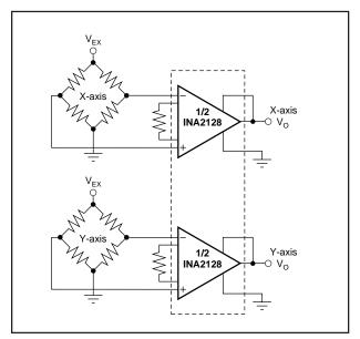
FIGURE 4. Two-Axis Bridge Amplifier.
