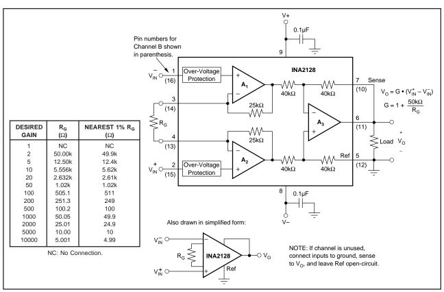
FIGURE 1. Basic Connections.
