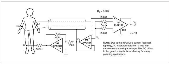
FIGURE 6. ECG Amplifier With Right-Leg Drive.
