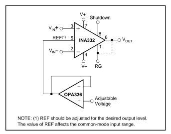
FIGURE 6. Optional Offset Trimming Voltage.
