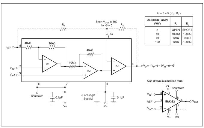
FIGURE 1. Basic Connections.
