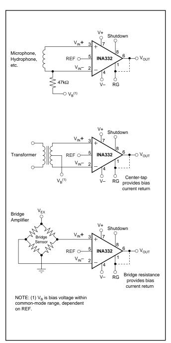
FIGURE 3. Providing an Input Common-Mode Path.
