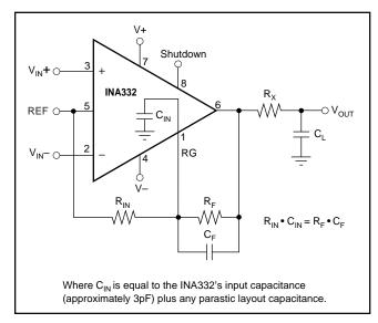
FIGURE 8. Feedback Capacitor Improves Dynamic Performance.
