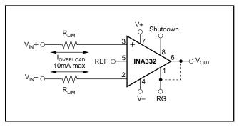
FIGURE 7. Sample Output Buffering Circuit.
