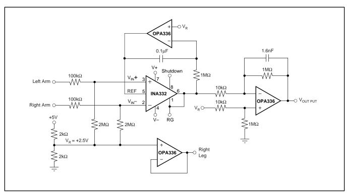
FIGURE 9. Simplified ECG Circuit for Medical Applications.
