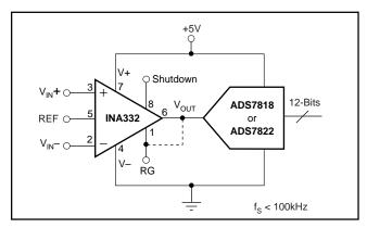
FIGURE 4. INA332 Directly Drives Capacitive-Input, High-Speed A/D Converter.
