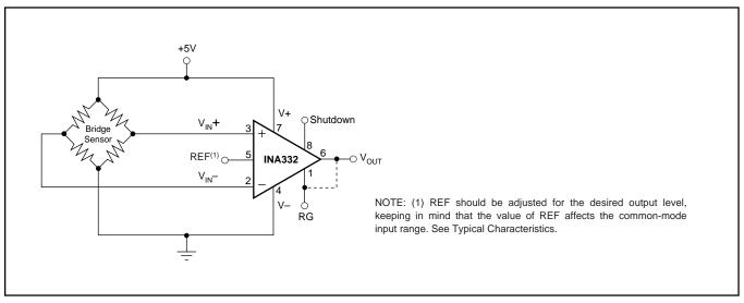
FIGURE 2. Single-Supply Bridge Amplifier.
