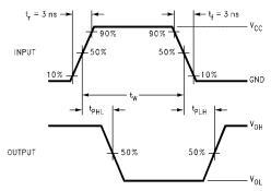
FIGURE 3. AC Waveforms
