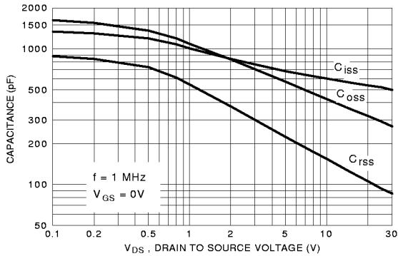
Figure 9. Capacitance Characteristics.
