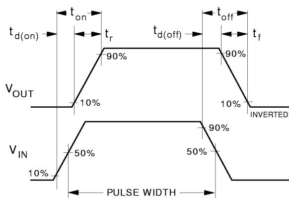
Figure 12. Switching Waveforms.
