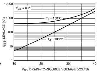
Figure 6. Drain-to-Source Leakage Current vs. Voltage
