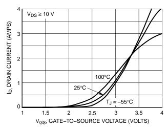
Figure 2. Transfer Characteristics
