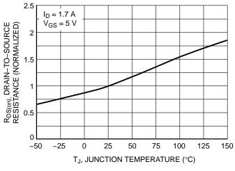
Figure 5. On–Resistance Variation with Temperature
