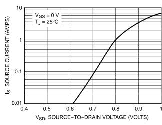
Figure 7. Diode Forward Voltage vs. Current
