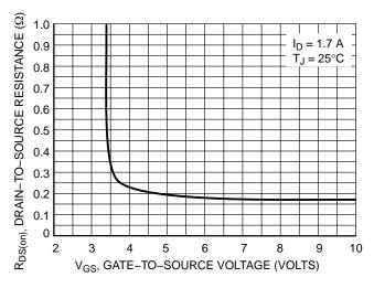
Figure 3. On-Resistance vs. Gate-to-Source Voltage
