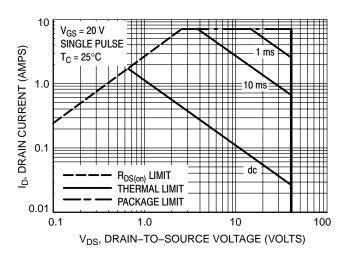
Figure 8. Maximum Rated Forward Biased Safe Operating Area
