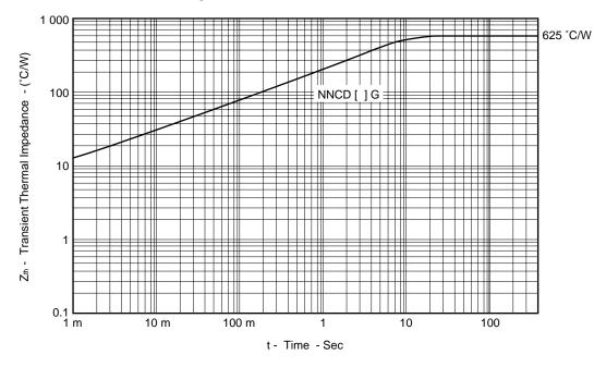
Fig. 4 TRANSIENT THERMAL IMPEDANCE
